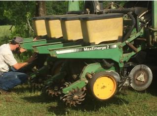
**Figure 2.** The no-till drill on the left has two hoppers so it can sow two cover crops at once (e.g., grass and a legume). In the photo on the right, note the coulters that are capable of opening a furrow.
